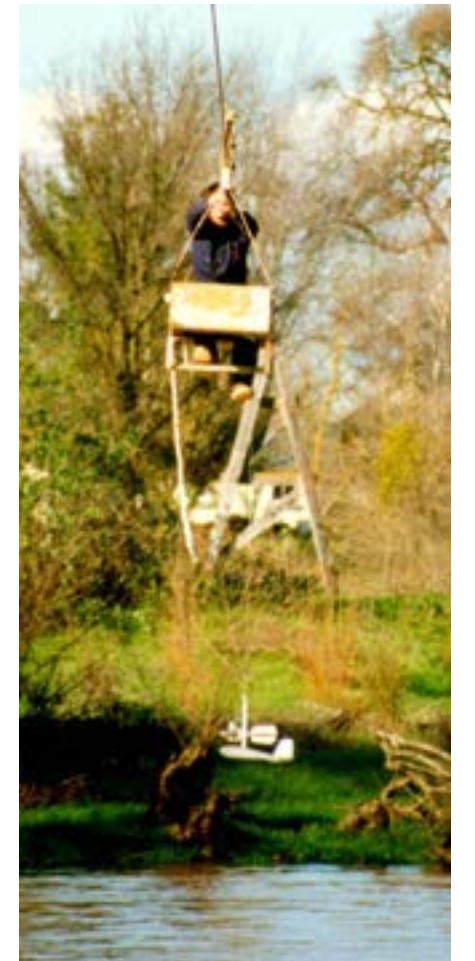
↑ Another means of measuring Kings River flows is utilized by a hydrologist riding a cable car and using this tool, dipped into the stream at various points, to calculate the volume of passing water.
